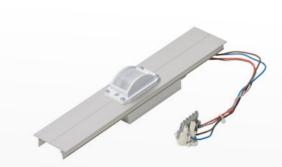
The waterproof Veko System Sensors are the ears and eyes of your lighting system. This simple plug & play solution can be used in combination with your DALI Pro or Encelium light management system. The Veko System Sensor has two versions: narrow and round. The required range determines which sensor you need. The Veko System Sensor is equipped with an extremely accurate infrared (PIR) sensor, which detects and interprets changes in the thermal image at lightning speed.
